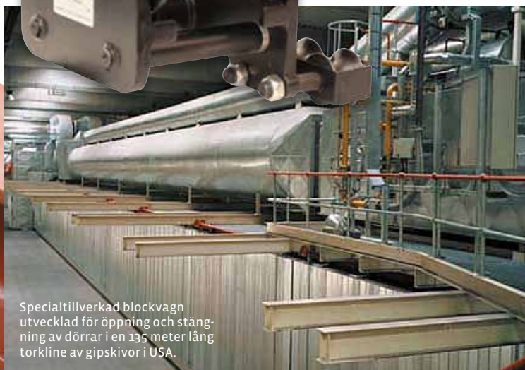
Customized Trolley developed for opening and closing of doors in a 135 meter long rail line for gypsum boards in USA.
