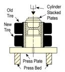
Now an easy way to press solid rubber tires. The TPP200 uses plates instead of combination rings to press a rim from an old tire into a new one. P They can be used on any Power Team press with 55 ton capacity or more.
