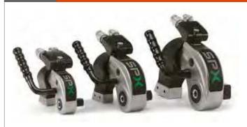
The tool's designed long-stroke mechanism imparts a minimum 30 degree nut rotation per stroke while maintaining a tight and compact nose radius. This is a clear advantage over the short stroke and back-up pawl mechanisms of light alloy competitive models. Fewer parts and reduced torsion in operation equals reduced wear, maintenance and associated costs.
