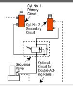
**Application**: Used when one cylinder in a multi-cylinder application must advance before any other.
