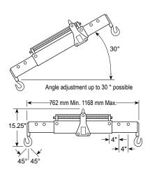
The working length is adjustable in three positions from 762 mm to 1168 mm. Maximum chain angle is 45  $^{\circ}$
