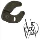
Designed to handle 51 to 152 mm dia. hydraulic cylinder gland nuts on many construction vehicles. Fits 6,4 and 7,9 mm dia. pin holes. Features a 3/4" sq. drive.
