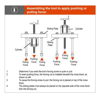
SELECTION AND CAPACITY RATING – Each Bi-Directional™ Puller's specified tonnage "capacity" is determined using its standard legs in tension. Using longer legs, or a setup in which the legs are in compression, will reduce the "capacity." Always select the largest "capacity" puller and the shortest legs that will fit the job.
