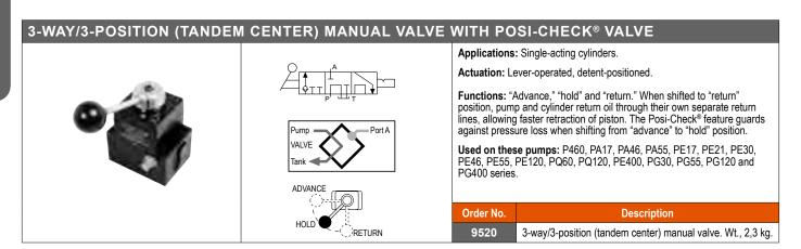
A CAUTION: To prevent sudden, uncontrolled descent of a load as it is being lowered, use a 9596 Load-Lowering Valve or 9720 Counter Balance Valve in conjunction with the directional valve used in your application.
