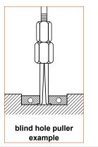
Removal of bearings, bushings, sleeves and other friction-fitted parts from blind holes can now be accomplished with ease. Set provides selection of expanding collets 8 to 44,5 mm I.D. Collet is placed through bore of part to be removed, then expanded with actuator pin so that lips of collet secure a positive grip for pulling. Pulling force is exerted by means of a forcing screw and bridge assembly or with a slide hammer. Equipped with a plastic case.
