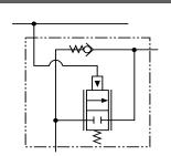
**Application:** Double-acting cylinders. Provides positive holding and controlled, "chatter-free" lowering of a load.
