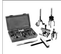
Components can be assembled to create several versatile puller versions. The puller head is turned to securely lock the jaws onto the part being removed. Both a 2-way and 3-way puller head are included, plus three long-reach and three short-reach puller jaws in a plastic storage box. Easily removes gears, bearings and other press-fitted parts.
