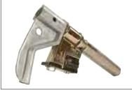
Restore damaged threads on shafts, housings, cages, etc., for re-assembly of matching parts. Eliminates need for thread-cutting equipment. Will not harm threads. V-pads and dies can be replaced. Cap. 32 to 127 mm O.D.
