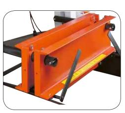
Width adjusts from 102 mm to over 686 mm; is secured with locking bolts.
