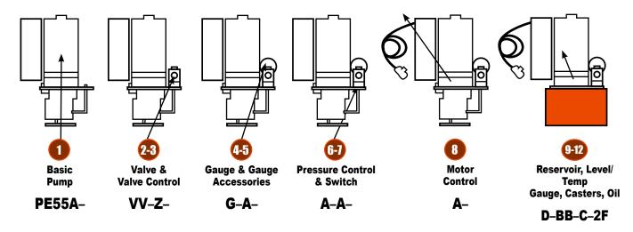
Pump No. **PE55A–VV–Z–G–A–A–A–D–BB–C–2F** is a 700 bar two-speed pump with a 115V, 50-60Hz, single-phase, 1,12 kW, 12000 rpm motor; a 9512 4-way solenoid valve with a 202778 remote hand control, a 9041 pressure gauge, no gauge accessories, standard pressure control, standard On/Off/Pulse motor control, 40063OR9 7,6 reservoir, a 350431 oil level/temperature gauge, 10494 casters, and 7,6 I of standard hydraulic oil.
