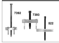
Ideal for pulling many small parts having tapped holes. The 7392 and 7393 may be used with the 1122 pulling attachment to remove bearings, etc. Pullers include two hex head cap screws, 3/8" – 16 NC x 76 mm long. Spread: 38 - 108 mm. Width of puller block is 124 mm. Cap screws are not included with the 522, but any cap screws up to 12,7 mm diameter may be used. The 522 spread, when used with 12,7 mm dia. cap screws, is 51 - 197 mm. Width of the 522 puller block is 209 mm.
