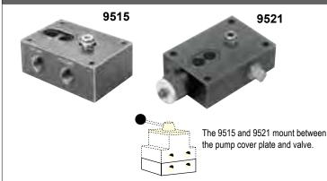
When fitted between pump cover plate, valve mounting flange, and control valve, provides a separate 3/8" NPTF female port, open to "return" regardless of position of valve. Also provides a separate 3/8" NPTF female pressure port. This sub-plate can be useful when you desire to use one pump with a deck-mounted control valve, plus a separate remote-mounted valve to control another function.
