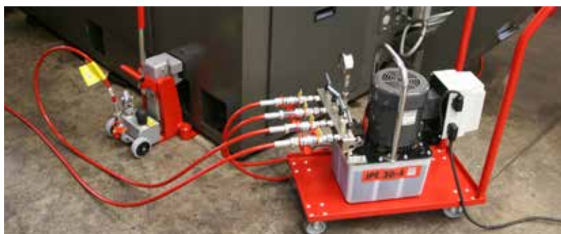
Electric pump JPE 30-NVR with 2 jacks in operation.
