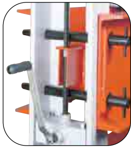
Lifting screw and locking pins make bolster raising a one-man job.
