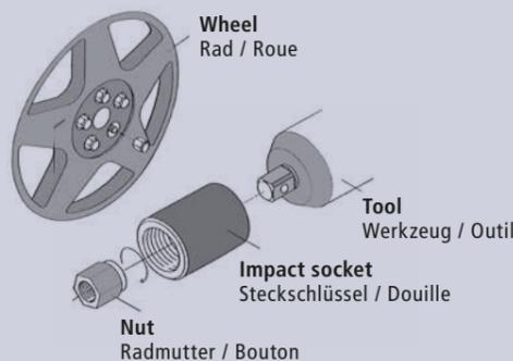
For removal of wheel lock nuts when special key is lost or not supplied upon service and for removal of the wheel nut when hexagon is damaged.
